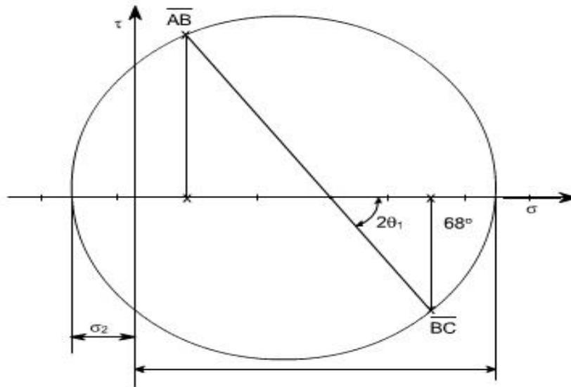
Taking the measurements from the Mohr's stress circle, the various quantities computed are
