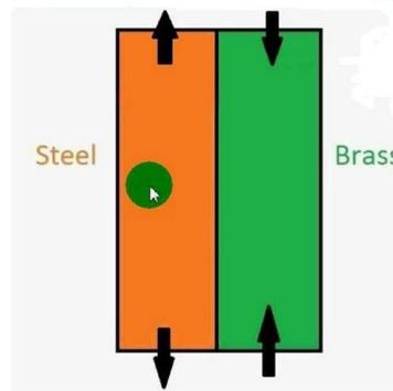
2. There will be free expansion or free contraction in the material according to the rising or lowering of temperature of the material.
