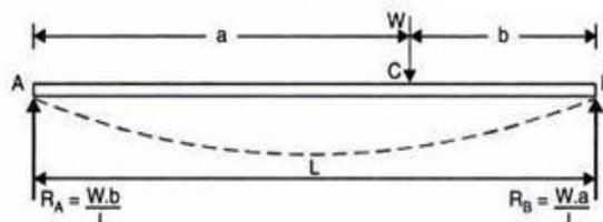
The bending moment at any section between A and C at a distance  $x$  from A is given by,
