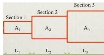
2. Length and cross-sectional areas of each section of bar is different and therefore stress induced, strain and change in length too will be different for each section of bar.
