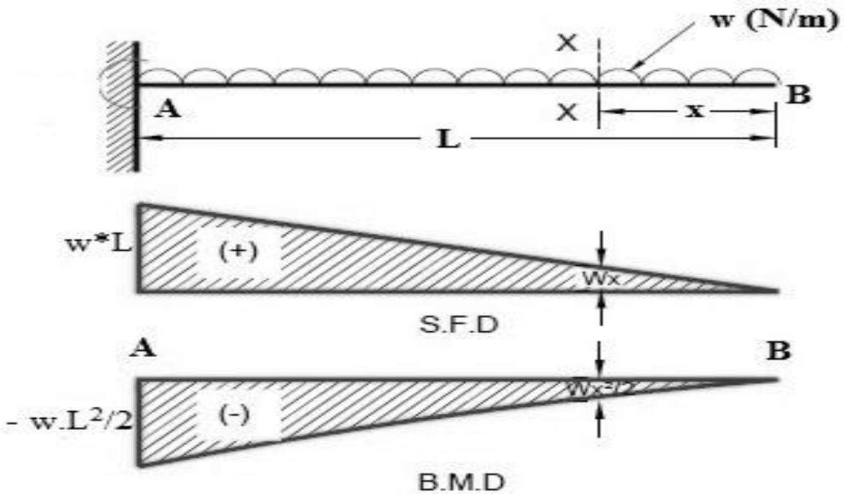
**SHEAR FORCE AND BENDING MOMENT DIAGRAM FOR CANTILEVER BEAM CARRYING UNIFORMLY VARYING LOAD**
