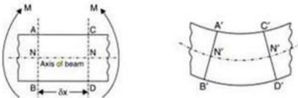
1. Consider a beam subjected to simple bending. Consider an infinitesimal element of length  $dx$  which is a part of this beam. Consider two transverse sections AB and CD which are normal to the axis of the beam and parallel to each other
