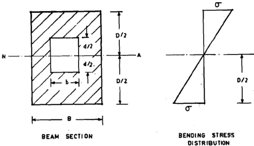
$$\begin{aligned} \therefore \text{Section modulus, } Z &= \frac{I}{y_{\max}} \\ &= \frac{1}{12} [BD^3 - bd^3] \times \frac{2}{D} \\ &= \left[ \frac{BD^3 - bd^3}{6D} \right] \end{aligned}$$
