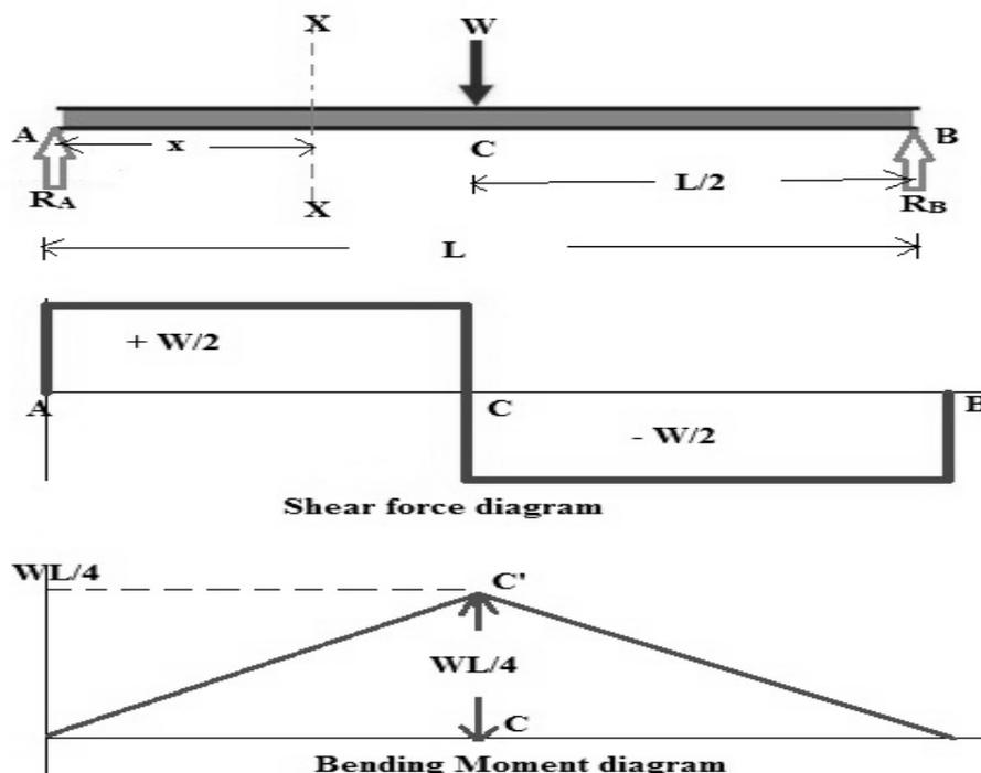
**SHEAR FORCE & BENDING MOMENT DIAGRAM OF A SIMPLY SUPPORTED BEAM CARRYING ECCENTRIC POINT LOAD :**
