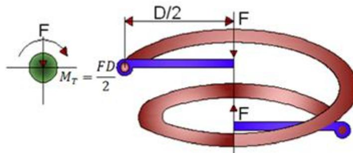
The cut sections of the spring, subjected to tensile and compressive loads respectively, are shown
