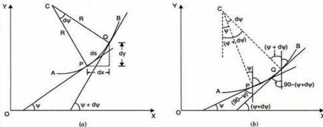
The point  $C$  is known as centre of curvature of the curve  $PQ$ .
