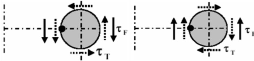
The broken arrows show the shear stresses arising due to the torsion  $T$  and solid arrows show the shear stresses due to the force  $F$ .
