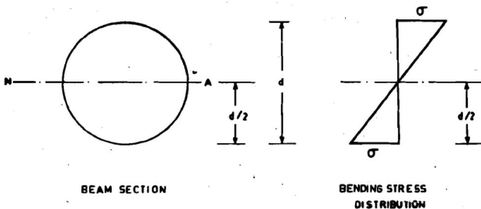
$$\begin{aligned} \text{Section modulus, } Z &= \frac{I}{y_{\max}} \\ &= \frac{\pi d^4}{64} \times \frac{2}{d} \\ &= \frac{\pi d^3}{32} \end{aligned}$$
