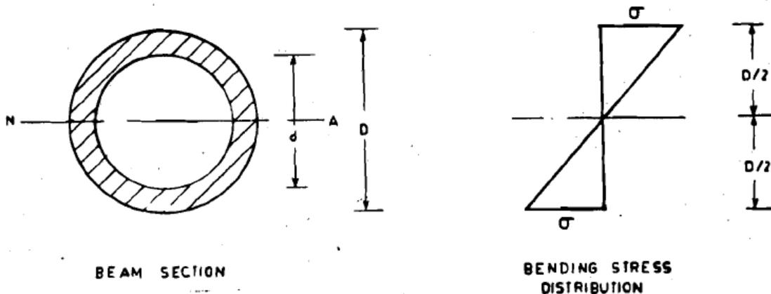
$$\text{Moment of inertia about the neutral axis, } I = \frac{\pi}{64} [D^4 - d^4]$$
