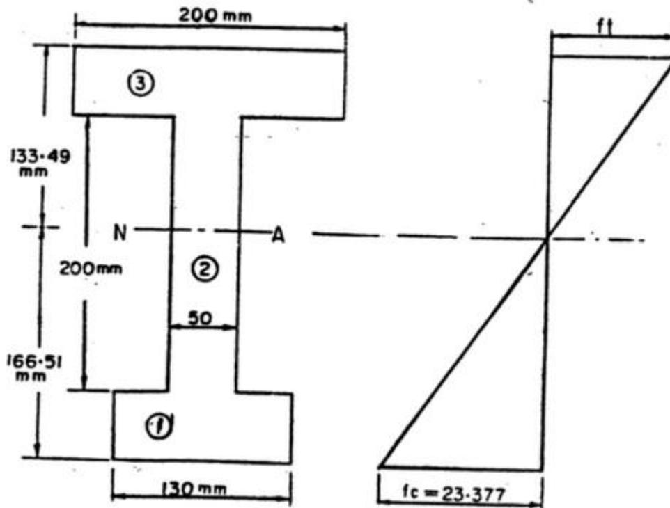
This stress will be compressive. In case of cantileers , upper layer is subjected to tensile stress, whereas the lower layer is subjected to compressive stress.
