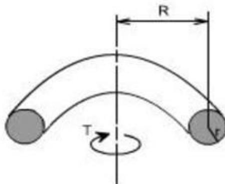
In this case the material of the spring is subjected to pure bending which tends to reduce Radius R of the coils. In this case the bending moment is constant throughout the spring and is equal to the applied axial Torque T. The stresses i.e. maximum bending stress may thus be determined from the bending theory.
